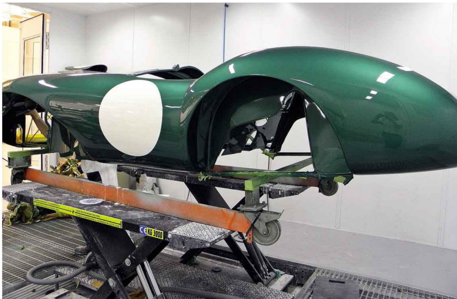
Clockwise from above Body gets its final coat of Aston Racing Green in the Works paint booths; steering gear and front and rear suspension components look so good after refurb it's a shame they're out of sight
