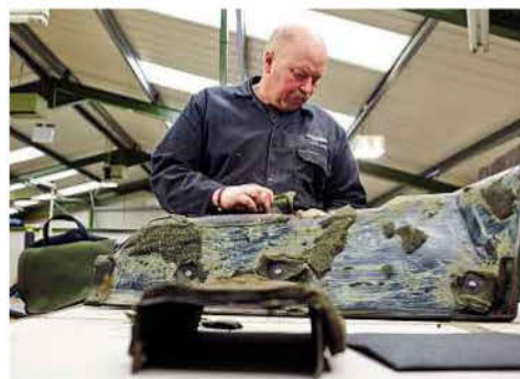
Clockwise from far left Stripped and shot-blasted chassis in the bodyshop's dedicated 'steel bay'; DB2 drophead and DB6 in the main workshop; trim specialist Colin Brown strips a transmission tunnel; and workshop manager John Gray outside the bodyshop's aluminium bay
